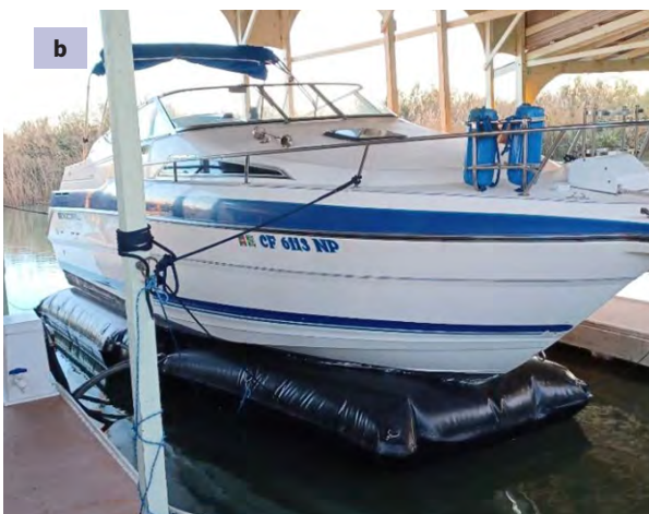
Figure 4.22 a) A motorized recreational boat suspended onto a floating system to prevent biofouling and b) the presence of biofouling on the structure
