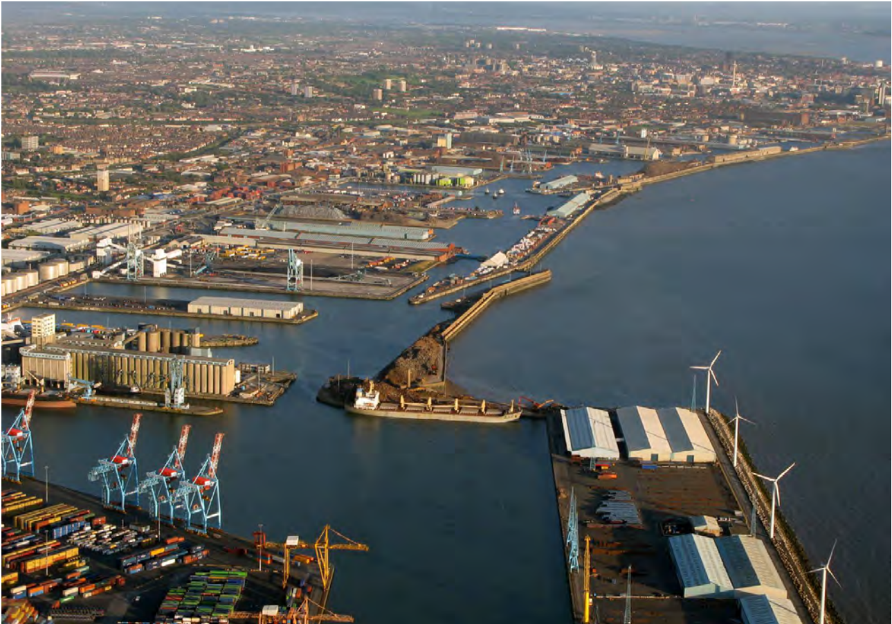
Figure 4.5 Typical wet dock port arrangement.
