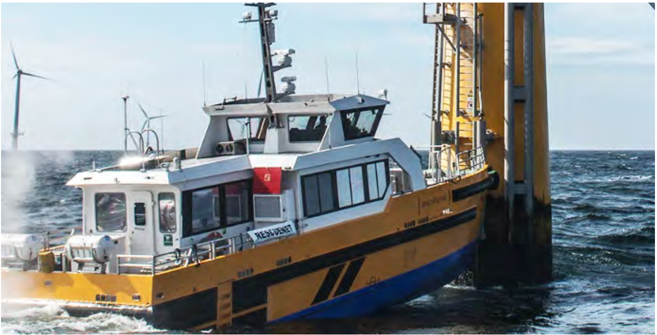
Figure 2.6 Windfarm service workboat and vertical access ladder. Note biofouling above the water line. Source: Windcats.
