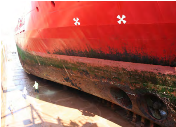
Figure 1.1 The microbial biofilm on a ship's hull provides a ready environment for the adhesion and growth of microalgae and bacteria.
