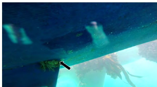
Figure 4.17 A recreational vessel with a relatively clean hull (depicted by the dark blue surface area) and biofouling in a niche area indicated by the joint between the hull and keel.
