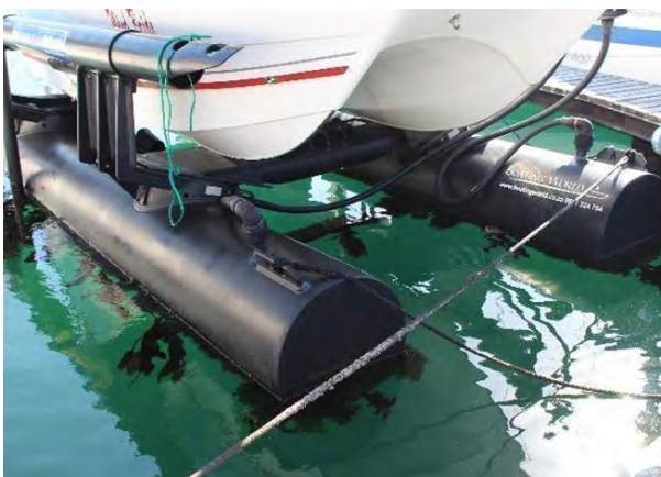
Figure 4.23 A motorized recreational boat suspended on a floating system to prevent biofouling.
