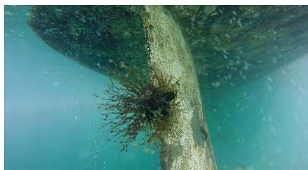
Figure 4.18 Biofouling on the rudder (niche area) of a vessel.
