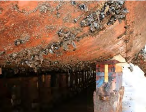
Figure A8 Niche areas: Bilge keels. Source: David Smith.
