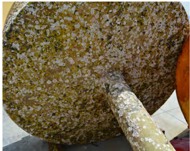
Figure 1.12 Monitoring buoy after being cleaned, showing remains of barnacles not removed by standard cleaning practices.
