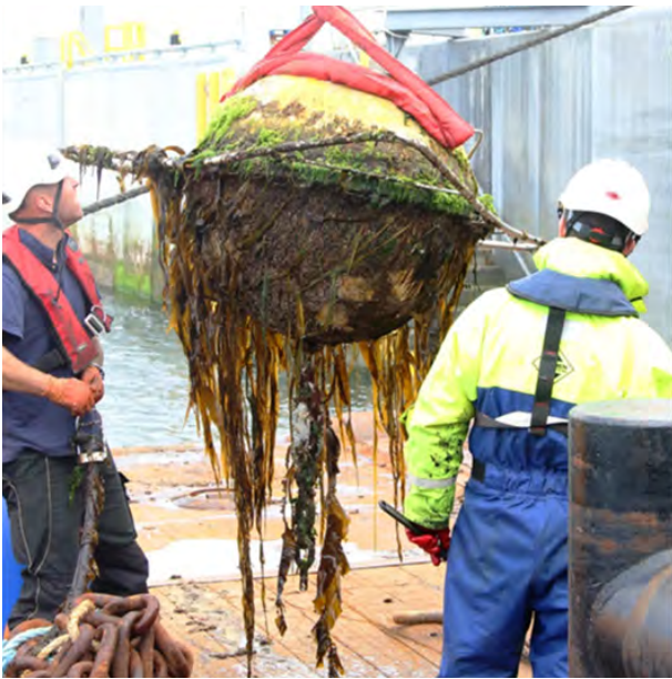
Figure 4.36 Fouling on a waverider buoy used to assess wave resource. Source: Want et al., 2017.
