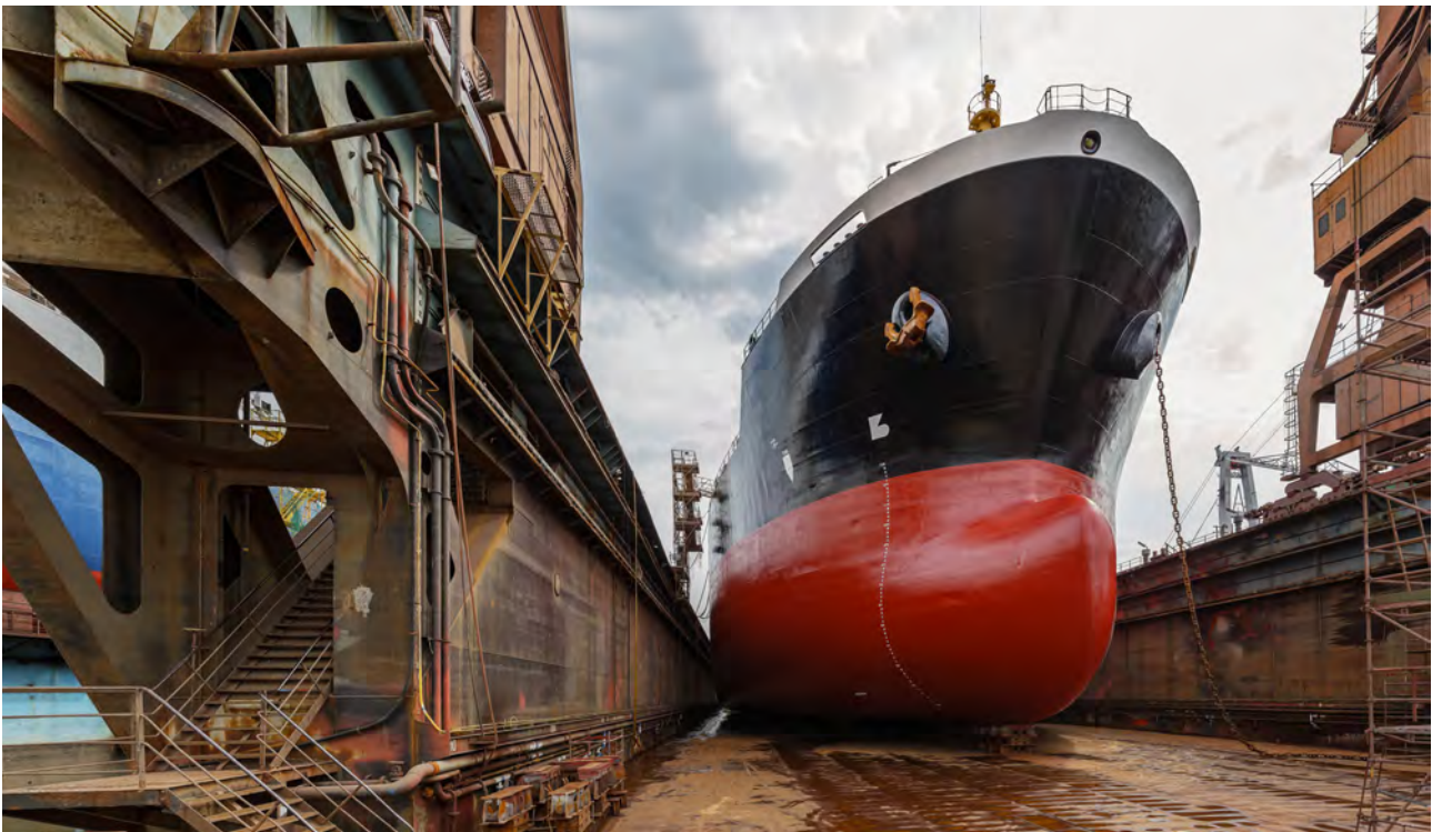
Figure 4.2 Large tanker hull designed for maximum cargo volume at slower speed have greater operating draft and considerably larger WSA when fully loaded. Source: Nightman1965/Shutterstock.
