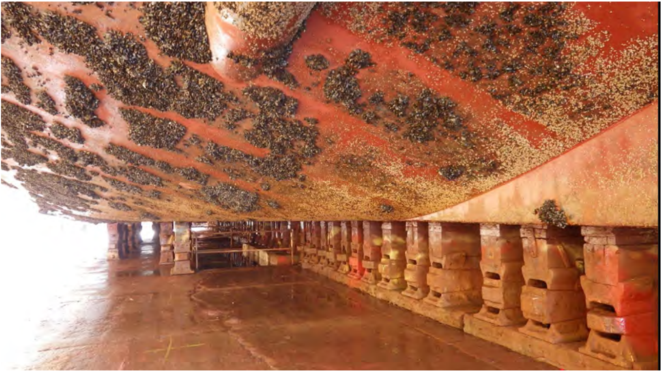
Figure 4.3 Underside of a ship's hull showing extensive fouling. Source: David Smith.
