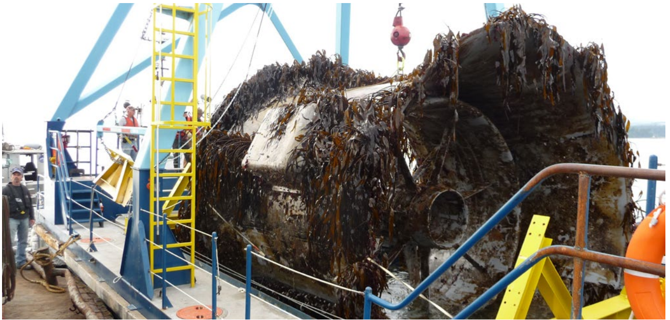
Figure 18. A tidal current turbine colonized by kelp after three years of immersion at the Race Rocks site, Canada. Source: Quillien et al., 2018.
